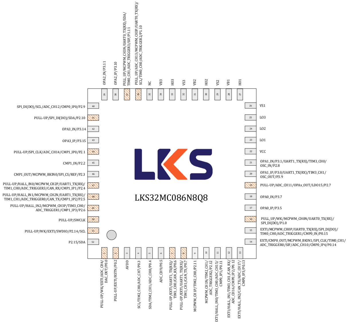
Fig. 3-2 LKS32MC086N8Q8(B) Pin Assignment
