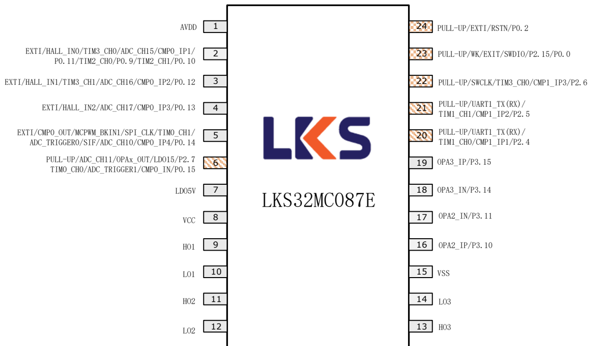
Fig. 3-2 LKS32MC087EM6S8 Pin Assignment
