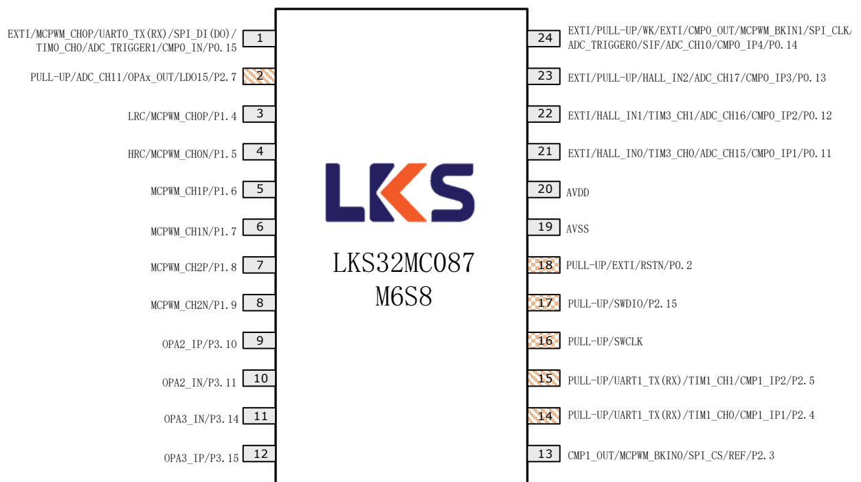
Fig. 3-6 LKS32MC087M6S8(B) Pin Assignment
