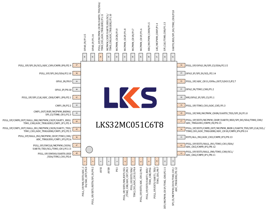
Fig. 3-1 LKS32MC051C6T8 Pin Assignment
