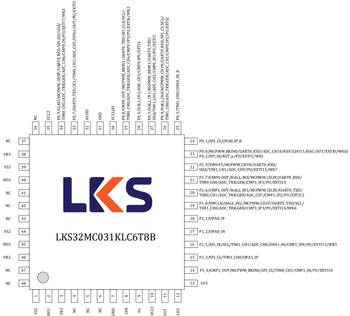
Figure 3-1 LKS32MC031KLC6T8B(C) Pin Assignment Diagram
