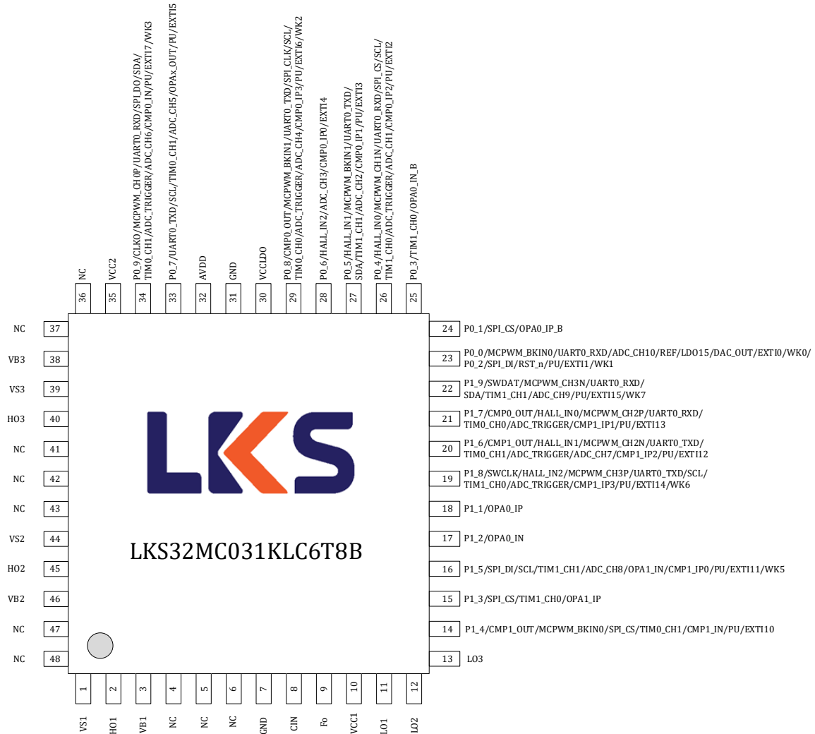
Figure 3-1 LKS32MC031KLC6T8B(C) Pin Assignment Diagram
