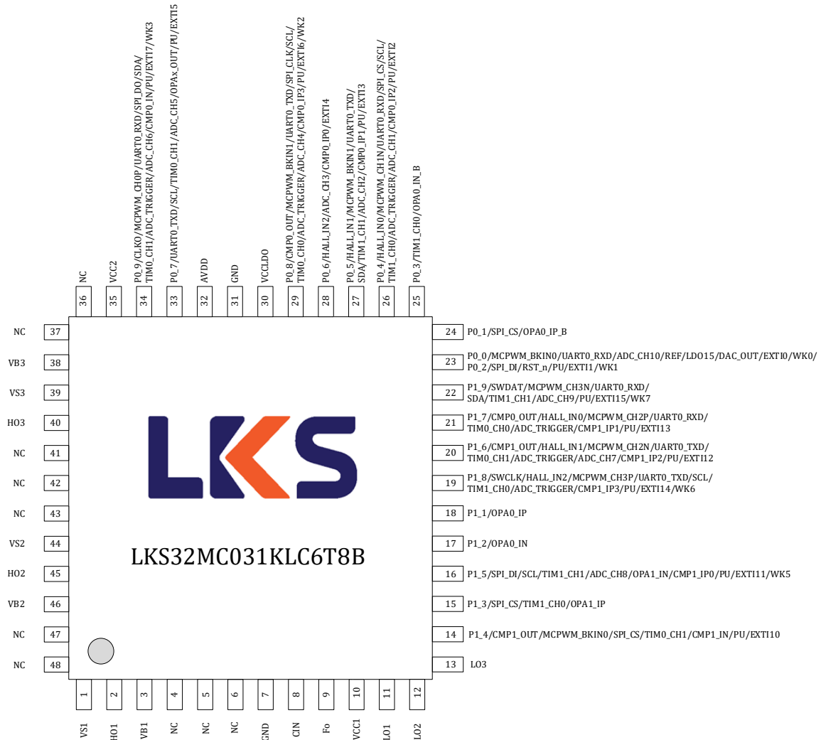
Figure 3-1 LKS32MC031KLC6T8B(C) Pin Assignment Diagram
